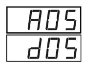
The set point for absolute value control is indicated by an "A" and the set point for differential control by a small "d" before the temperature value. The absolute value control temperature can be set between 2 to 15 °C [35.6 to 59 °F]. The differential value control temperature can be set between dT = 2 to 15 °C [dT = 3.6 to 27 °F].
