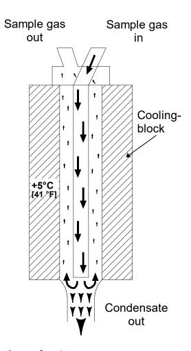
Figure 4 Diagram of the heat exchanger function
