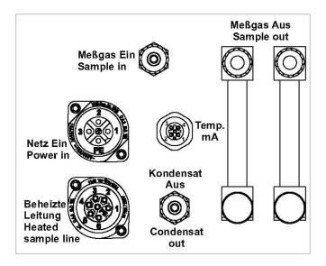
Figure 2 Labelling of the connections
