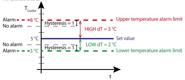
Figure 11 Temperature alarm limits and hysteresis
