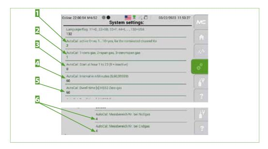
Fig. 87: Activating AutoCal and entering parameters
