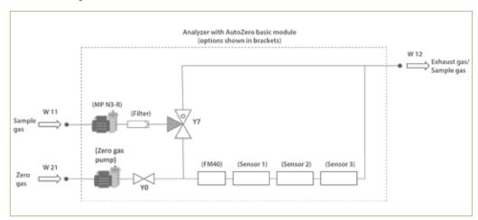
Fig. 93: AutoZero basic module with options
