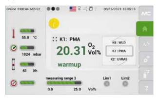
Fig. 37: M2/S2 - Detailed view during warm-up period
