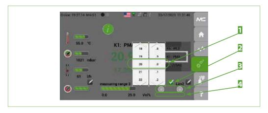
Fig. 47: Highlighted scroll bars to set operational parameter Lim1
