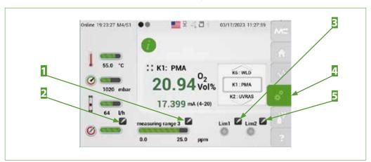
Fig. 44: M4/S1 Edit buttons for measuring range and operational parameter settings
