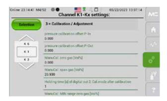
Fig. 76: Setting the channel-specific calibration parameters
