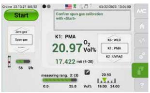
Fig. 77: Manual calibration with span gas
