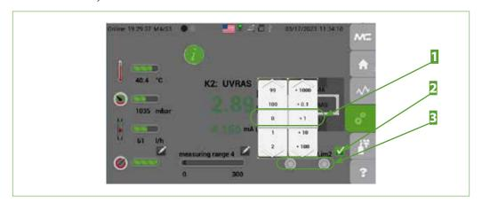
Fig. 48: Highlighted scroll bar to set operational parameter Lim2
