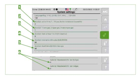
Fig. 95: AutoZero: activate AutoCal procedure and select zero gas
