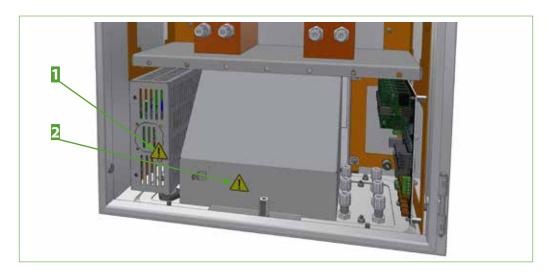
Fig. 4: Warning symbols inside wall-mount housing
