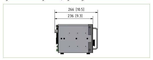
Fig. 12: 19"-rack housing side view (short housing)
