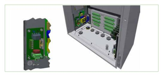
Fig. 16: Power supply connections inside wall-mount device (w/o protective covers)
