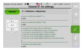
Fig. 98: mA setting: Page M4/S2, 3=Calibration/Adjustment
