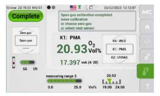
*Fig.* 81: End of the manual calibration procedure
