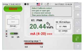
Fig. 83: A terminated manual calibration procedure
