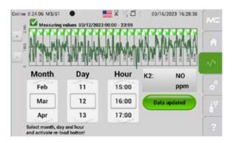
Fig. 82: Data logger screen with green calibration symbols
