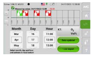
Fig. 85: Datalogger screen with red calibration symbol
