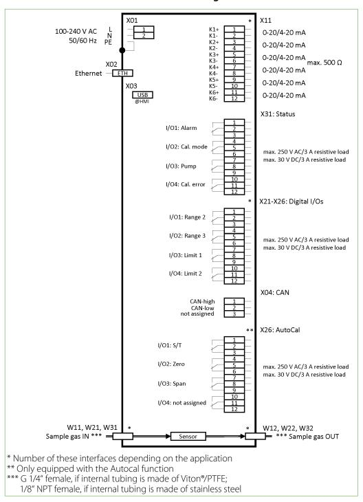
Fig. 20: Electrical interfaces: wall-mount housing
