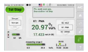
Fig. 78: First step of the manual calibration procedure
