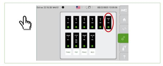
Fig. 88: Diagnostic diagram: Opening the output card "IOAC 0" of channel K2
