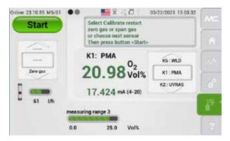
Fig. 97: AutoCal start without setting the interval: Channel selection
