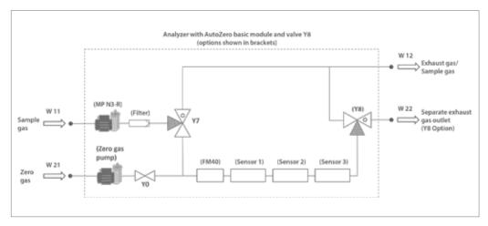
Fig. 94: AutoZero basic module with 3/2 way valve Y8 (optionally)
