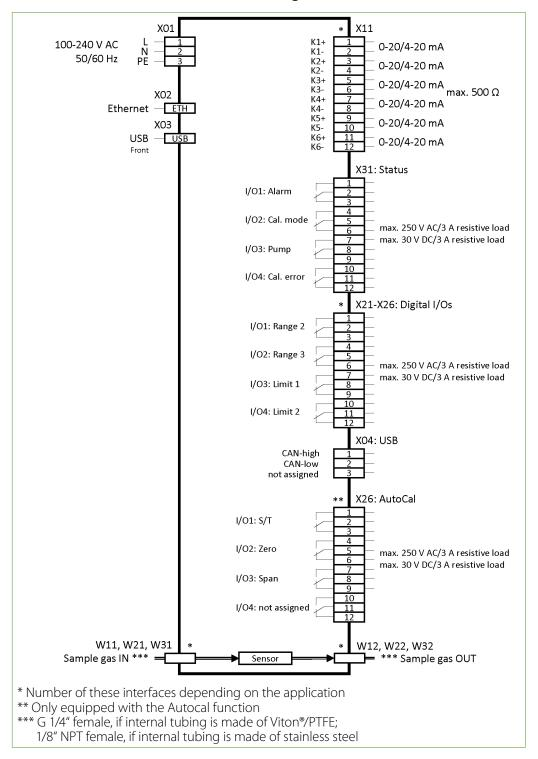
Fig. 19: Electrical interfaces: 19"-rack housing
