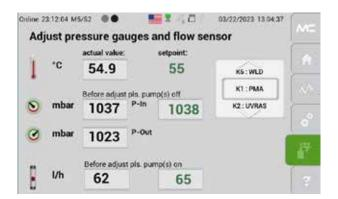
Fig. 71: Adjust pressure gauges and flow sensor
