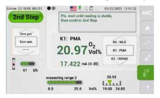
Fig. 79: Second step of the manual calibration procedure
