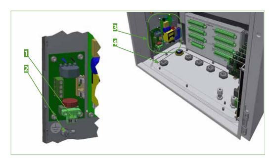
Fig. 72: Power supply connections inside wall-mount housing
