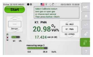
Fig. 70: Gas calibration screen
