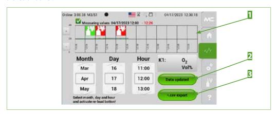
Fig. 42: M3/S1 - Recorded data selection screen
