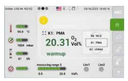
Fig. 73: Warm-up phase in M2/S1 and warm-up info on M2/S2
