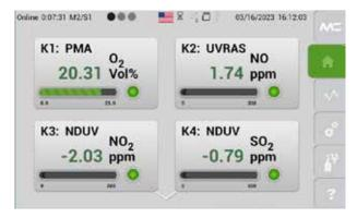
Fig. 21: Startup screen of the 6-Channel configuration
