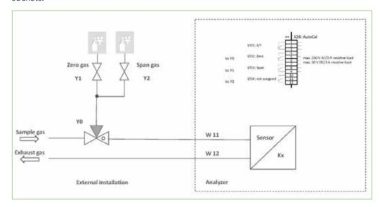
Fig. 90: AutoCal extern. valves: zero and span gas via gas cylinder
