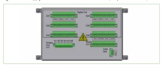
Fig. 17: Signal connections inside wall-mount device (max. equipped)
