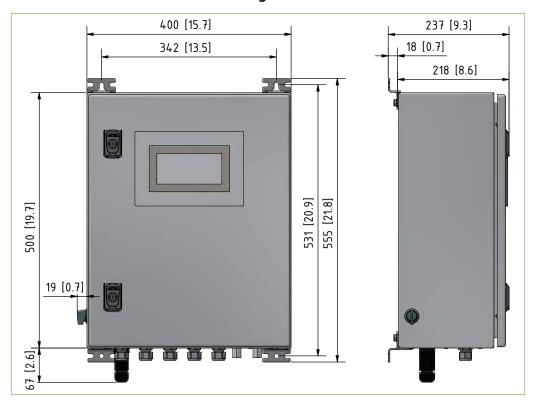
Fig. 13: Wall-mount housing, front and side-view
