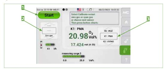
Fig. 96: AutoCal-Start without setting an AutoCal interval
