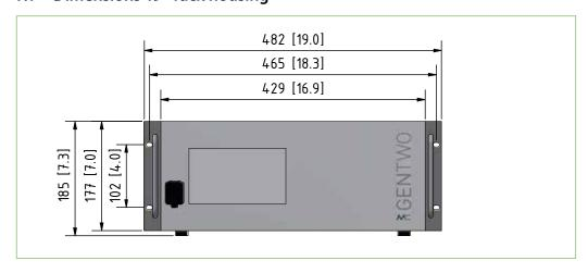
Fig. 10: 19"-rack housing front view
