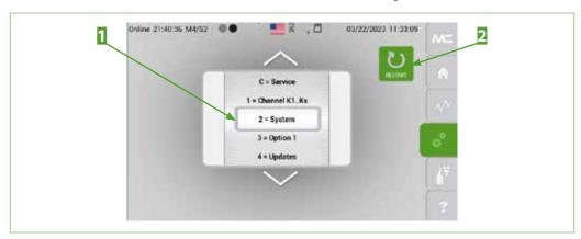
Fig. 49: M4/S2 screen with "Restart" button
