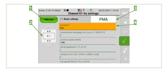
Fig. 51: Basic settings for channel 1
