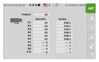
Fig. 33: M1/S4 - Operating hours counter (OHC)
