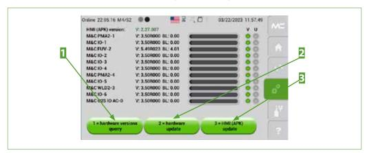
Fig. 56: Buttons to get information and install hardware and software updates
