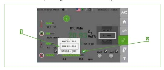
Fig. 45: Highlighted scroll bar to select measuring range
